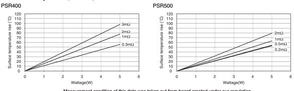
Measurement condition of this data was taken out from board created under our regulation. Product with highest temperature was selected for the measurement.
